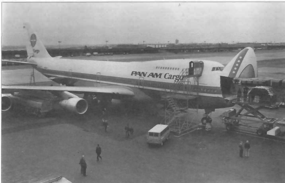
The nose-loading all-cargo 747F was capable of carrying nearly 100 tons of freight, including such large items as printing presses, drilling rigs and luxury limousines.
